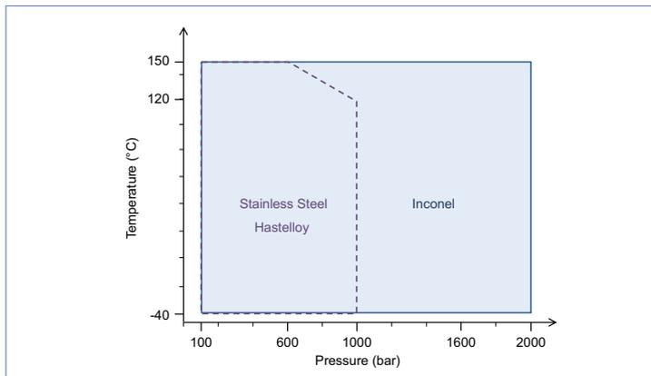
KELLER 6LHP series high-pressure transducers are available with various material options. Stainless steel, Hastelloy C-276, Inconel 718 or titanium can be selected (see "Mechanical data") in line with requirements.
