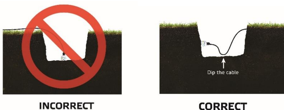
Figure 2.7 Horizontal placement sensor and dipping the cable is recommended
