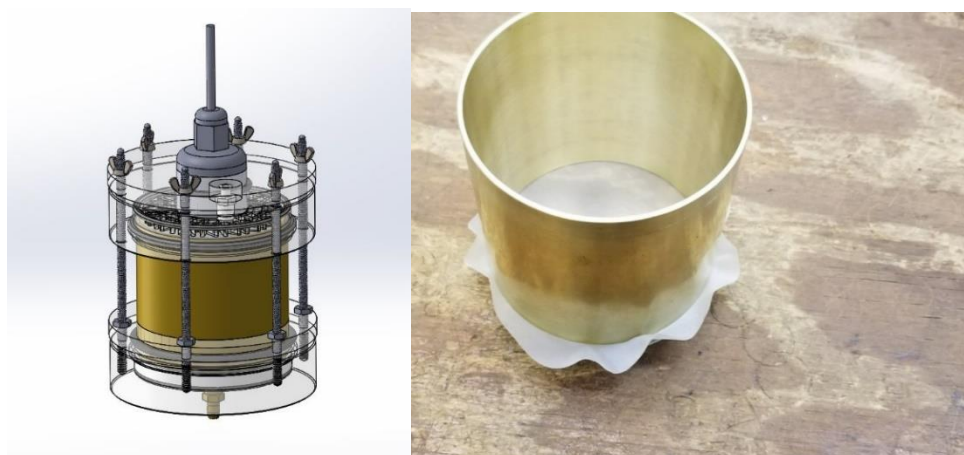
Figure 1.2A. The Tempe Cell for custom calibrations, soil water retention curve
