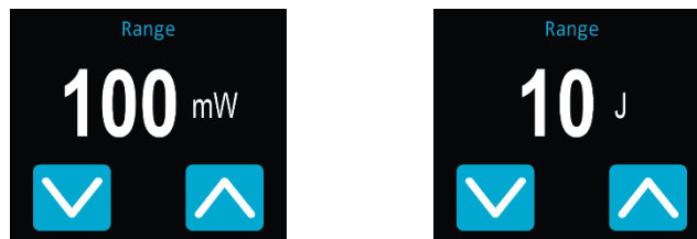
Figure 4. Up and down buttons to set the manual range or to go back to the default "Auto" range setting
