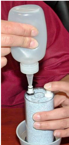
Figure 27 Checking desiccant for leaks
