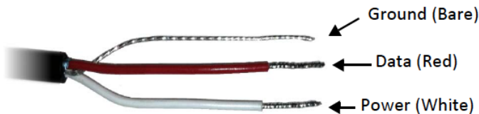
Figure 3: Pigtail End Wiring
