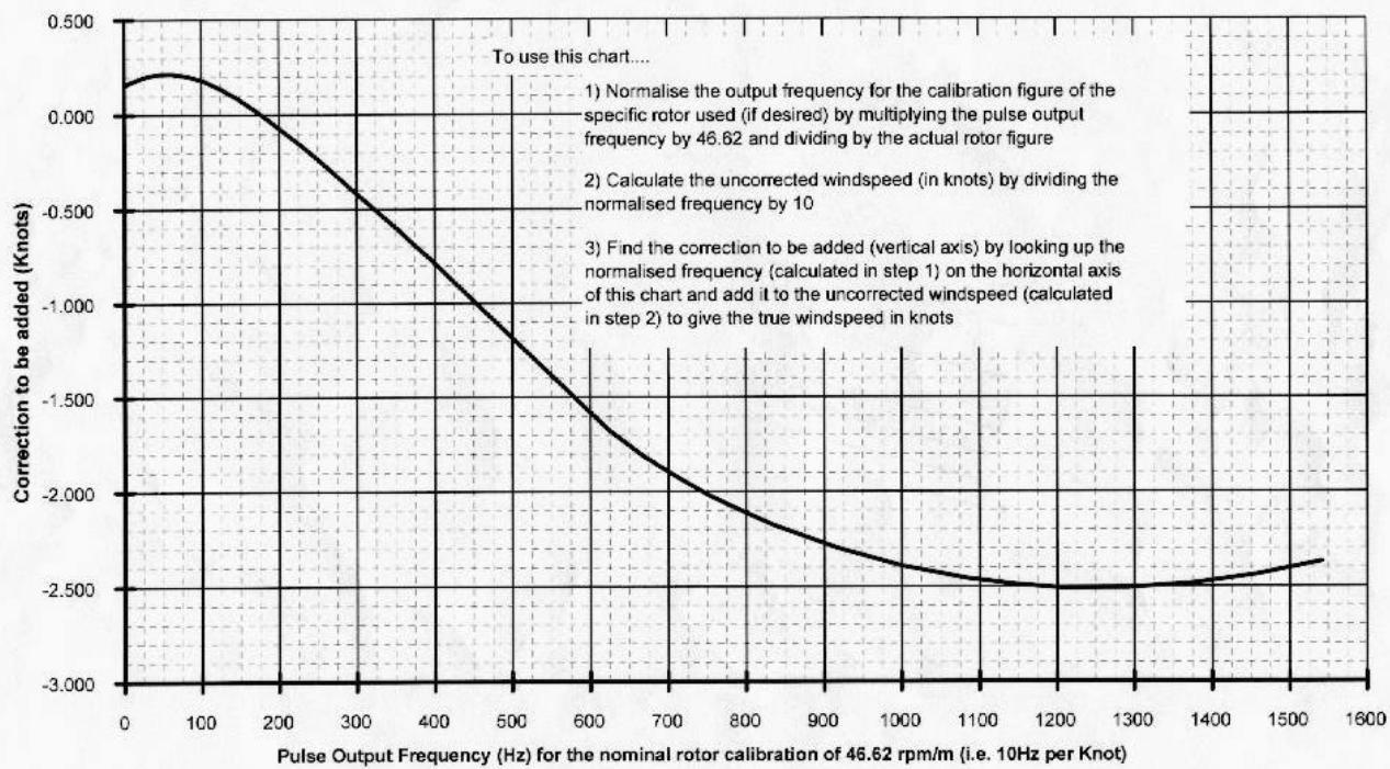
***Correction of Analog output of A100L2 for combined effects of
