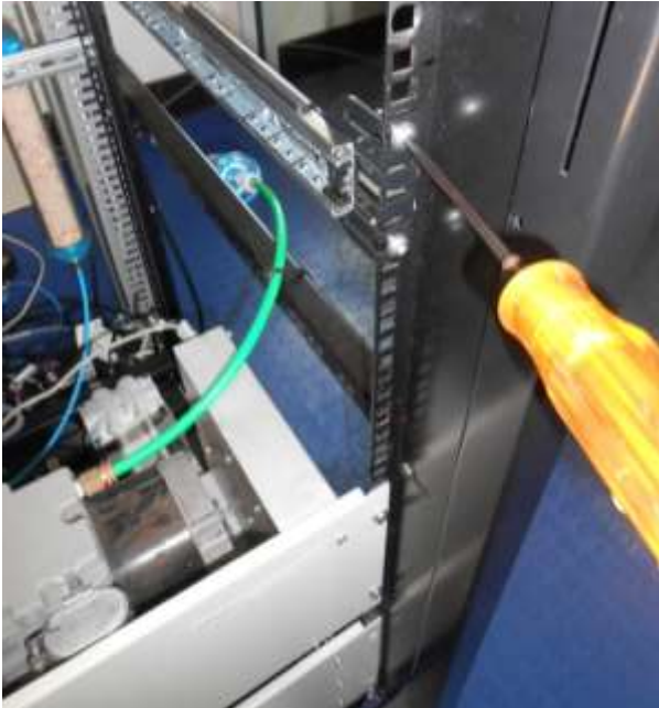
Figure 102 – Attach Slides to Front of Rack
