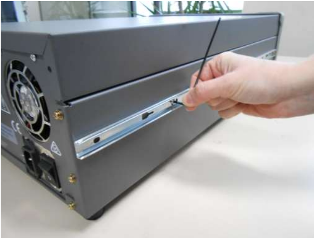
Figure 98 – Assemble Inner Slide on Chassis
