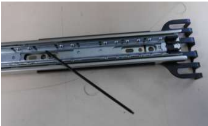
Figure 100 – Attach Rack Mount Adaptors to Outer Slides
