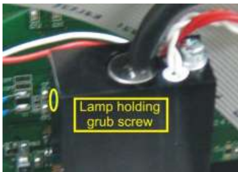
Figure 95 – Location of UV Lamp Fastening Grub Screw
