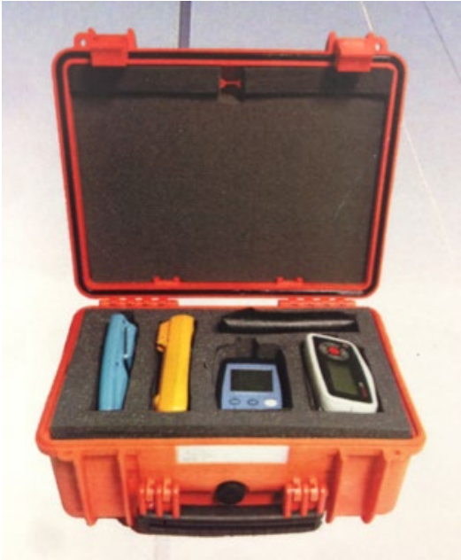
Figure 72 – Air Monitoring Test Equipment Kit (AMTEK) – Customisable
