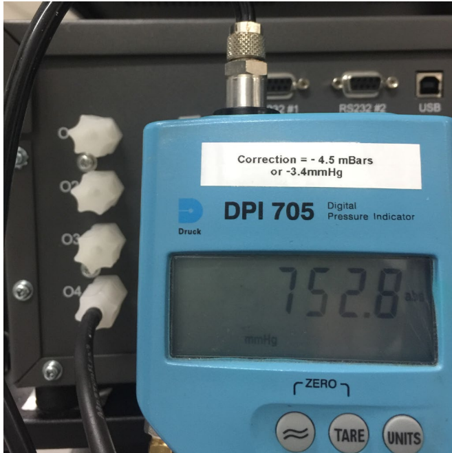
Figure 67 – Connecting the Barometer to O4 (Output 4)
