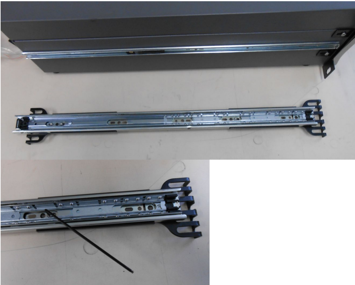
Figure 70 – Attach Rack Mount Adaptors to Outer Slides
