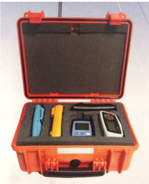
Figure 54 – Air Monitoring Test Equipment Kit (AMTEK) – Customisable
