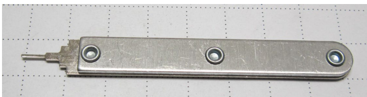
Figure 50 – Minifit Extraction Tool – (PN: T030001)
