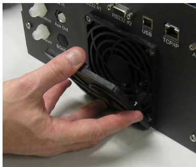
Figure 56 – Removing the Fan Filter
