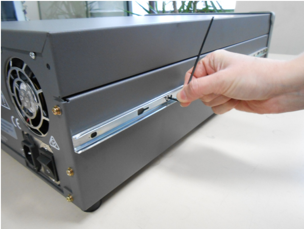
Figure 68 – Assemble Inner Slide on Chassis
