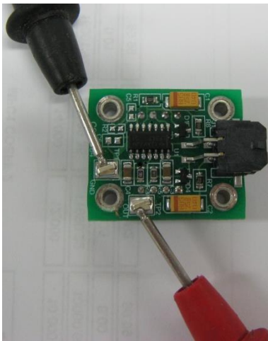
Figure 61 – Test Point Location
