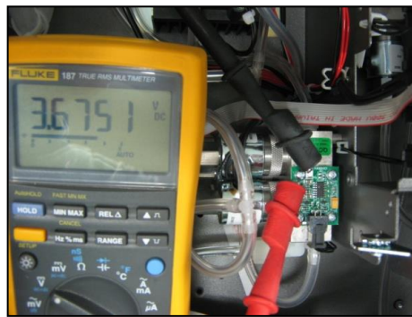
Figure 149 – Typical Test Point Reading of Cell Pressure Sensor
