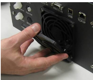
Figure 55 – Removing the Fan Filter
