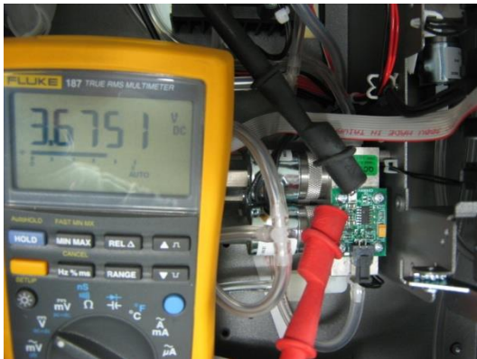
Figure 58 – Typical Test Point Reading of Measurement Cell Pressure Sensor
