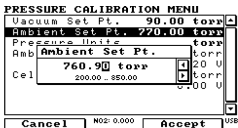
Figure 44 – Setting the Ambient Set Point
