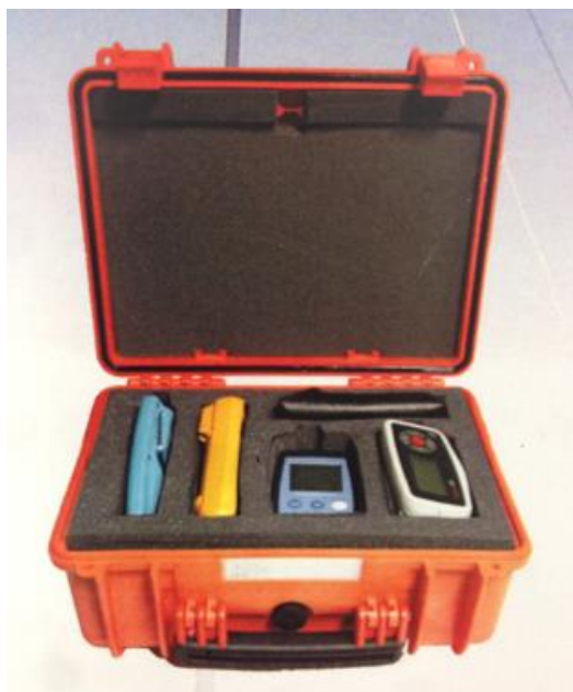
Figure 51 – Air Monitoring Test Equipment Kit (AMTEK) – Customisable
