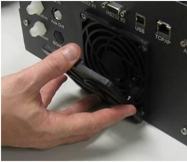
Figure 53 – Removing the Fan Filter
