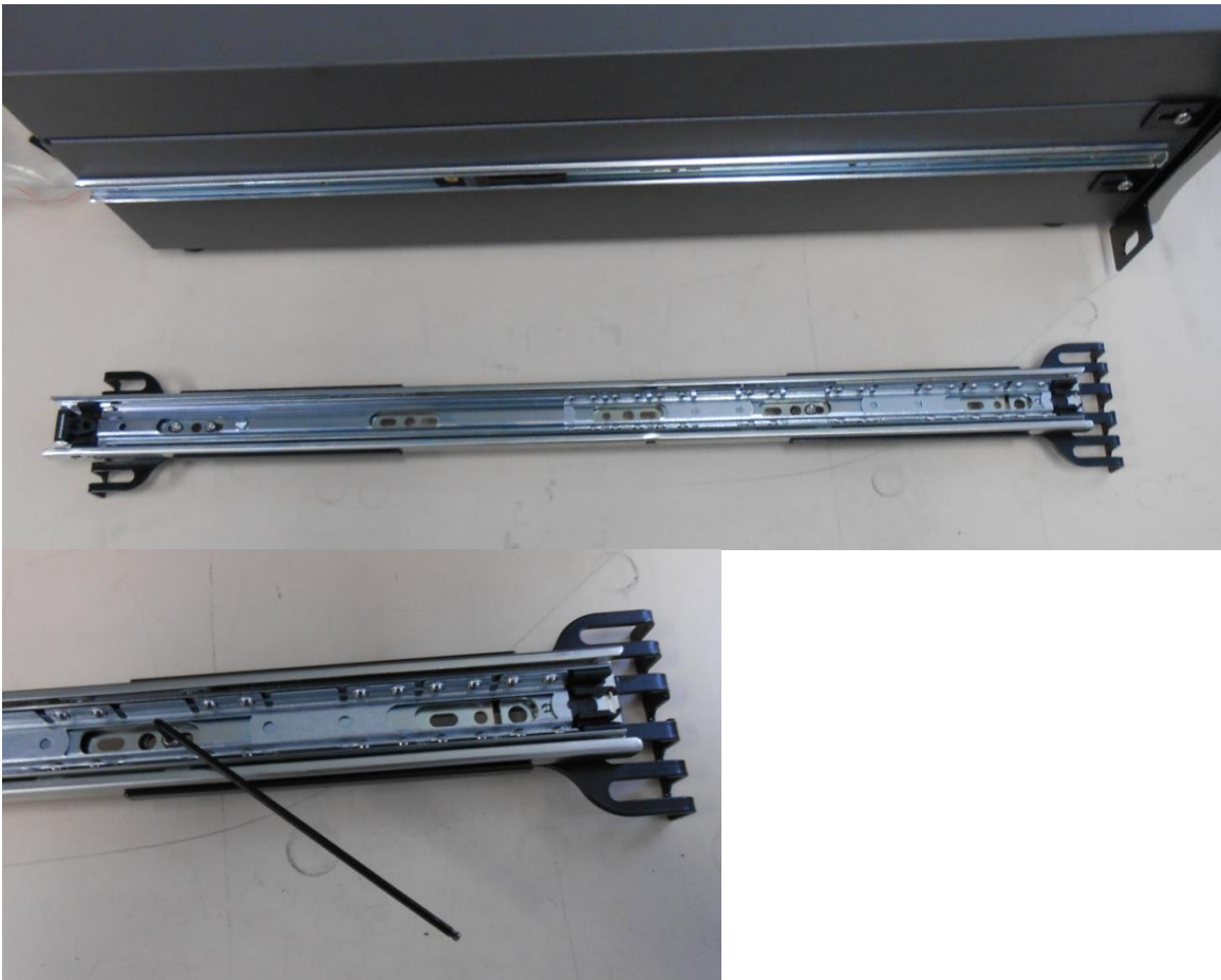
Figure 70 – Attach Rack Mount Adaptors to Outer Slides
