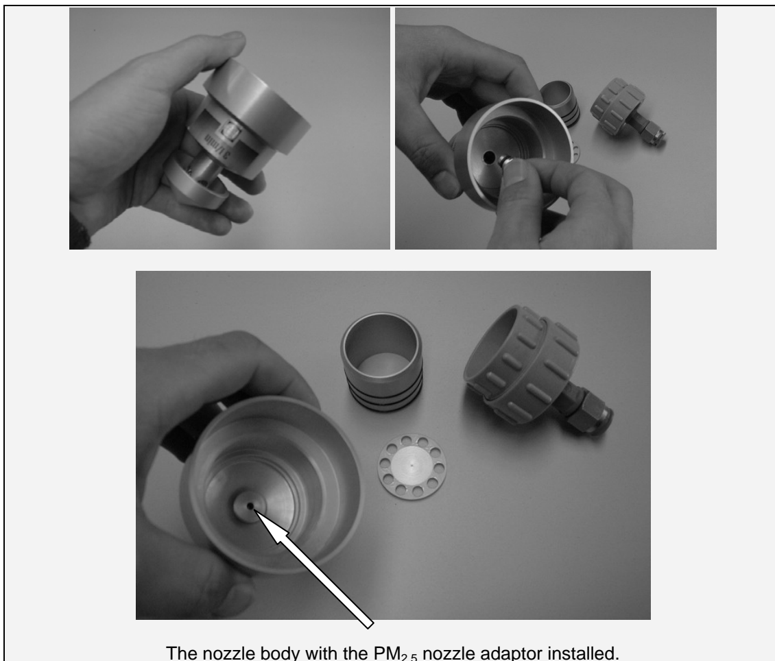
Figure 32 PM 2.5 Nozzle components and assembly
