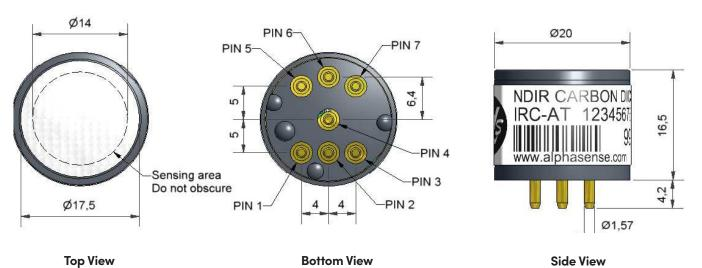
Dimensions are in millimetres (± 0.15mm).
