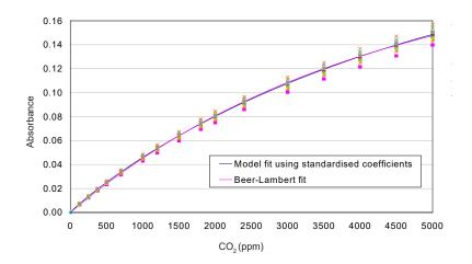
Typical response from 0 to 5000ppm CO<sub>2</sub>. The fit is very close to the theoretical curve, predicted by the Beer-Lambert Law.
