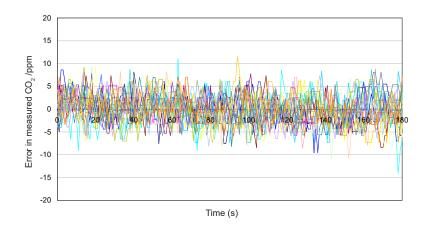
Excellent resolution and noise at 1000ppm  $CO_2$  for the IRC-AT is achieved by better design, not by using more expensive components.
