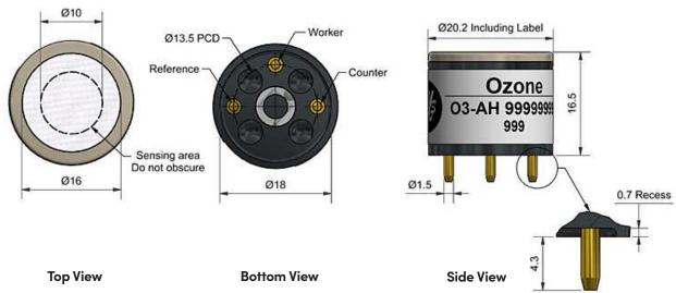
Dimensions are in millimetres (± 0.15 mm).
