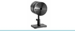
The BT50A-15 absorbs a laser beam that is inserted into the entrance aperture parallel to the unit's optic axis. The beam trap is designed that only a very small fraction of the light is backscattered. The BT50A-15 does not measure power. It is a beam trap only.
