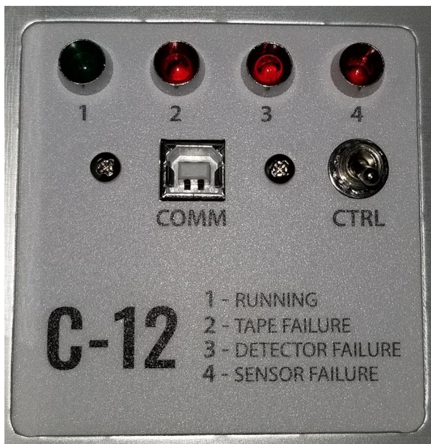
Figure 3-4 LED and Toggle Switch Interface
