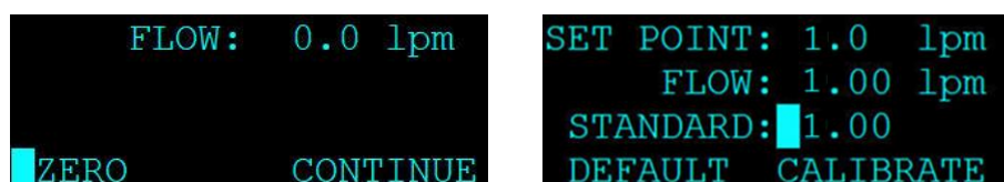
Figure 6-14 C-12 Calibrate Flow Screens
