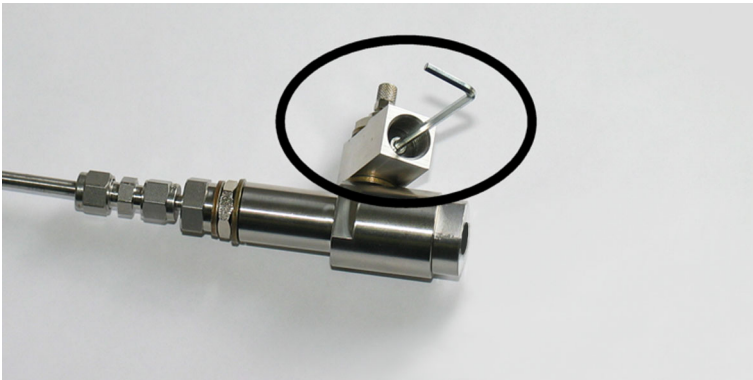
Figure 14 Removing the leak screw
