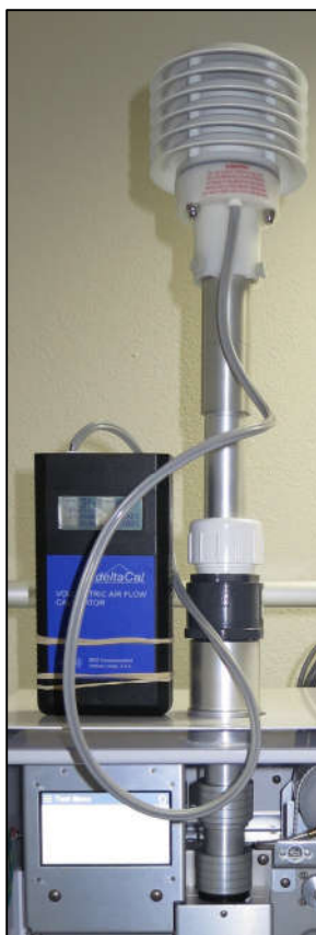
Figure 6-14 Installing the CTS on the Main Sample Inlet
