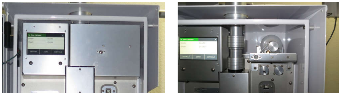
Figure 6-10 Flow System Cover Removed
