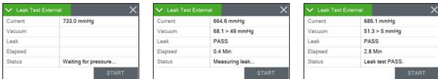
Figure 6-3 External Leak Test Sequence
