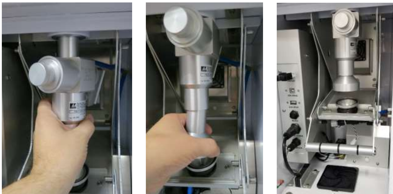
Figure 3-7 Installation of the PM 2.5 Cyclonic Separator
