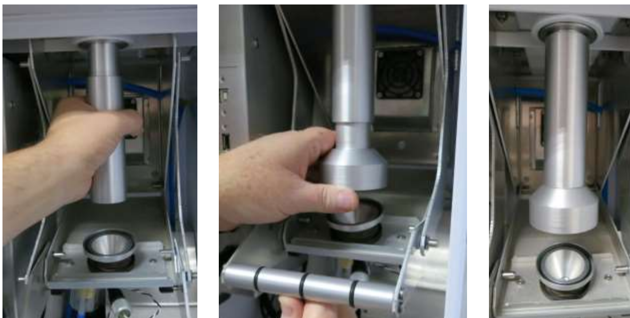
Figure 3-8 Installation of the PM 10 Pass-Through Adapter
