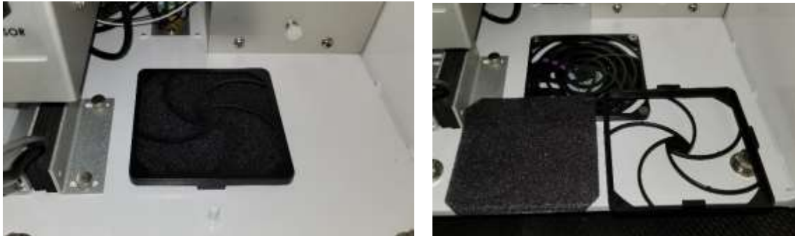
Figure 3-13 Dust Filter Installation
