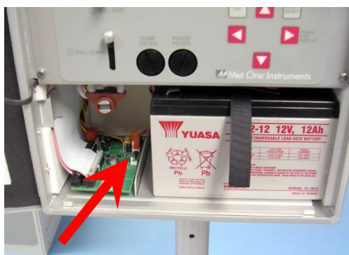
Internal battery and 81220 PCB battery harness connection
