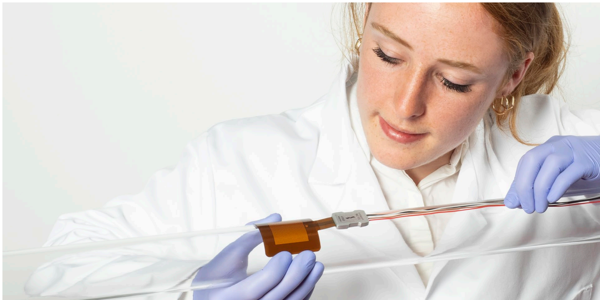
Figure 0.2 Application example: FHF04SC being installed to measure heat flux on a pipe
