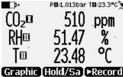
Figure 4 Display example with carbon dioxide and temperature and humidity probes connected simultaneously
