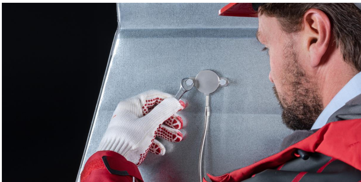
Figure 4.1.1 Example of an IHF02 industrial heat flux sensor mounted on an object to be measured using spring-loaded bolts. The sensor is mounted on a well prepared flat surface.
