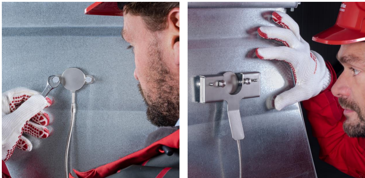
Figure 0.2 IHF02 industrial heat flux sensor mounted on an object using spring-loaded bolts (on the left), and with IHF02's easy-to-use optional magnet frame (on the right). The instrument is suitable for long-term use at one location as well as for survey purposes at multiple locations, also outdoor.
