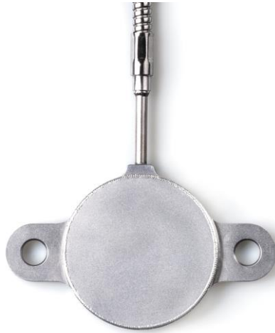
Figure 5.1.1 IHF02 showing its two flanges allowing installation on tack-welded M6 threads or with spring-loaded bolts (not included with IHF02). IHF02 should be mounted on a well-prepared flat surface
