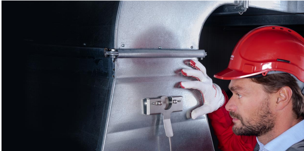
Figure 5.2.1. IHF02 industrial heat flux sensor mounted on an object using its optional magnet frame
