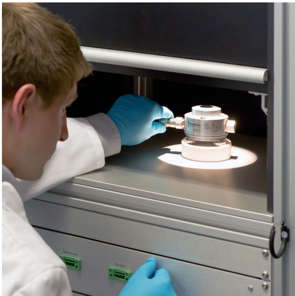
Figure 4 pyrometer during conformity assessment
