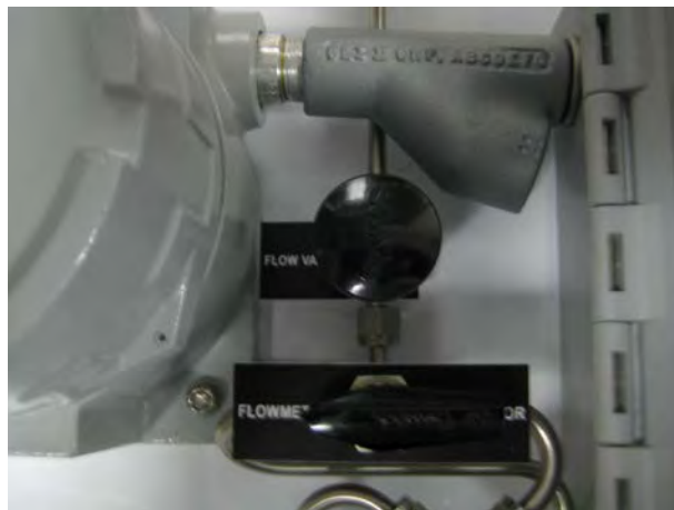
3-way Sample/Sensor valve and sample flow control needle valve
