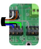
Using DeltaLINK version 3 or later configure channel 6 by choosing "ML3" and channel 7 by choosing "ML3 Temperature" from the sensor menu.
