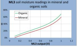
Note: The ML3 has been optimised for a 0.5 to 1 second warm-up period. Do not power the sensor continuously.
