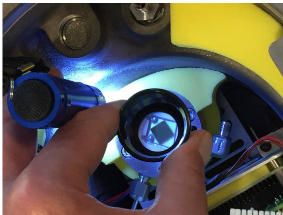
Figure 44 Checking the Mirror Surface
