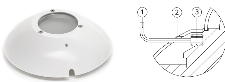
Figure 5.2.1 SCR01 sun screen and its installation and removal: turn the set screw using the hex key and lift off the sun screen to remove. (1) hex key, (2) sun screen, (3) set screw
