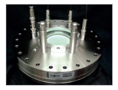
The Vacuum Imaging Detector (VID) for Ions and Electrons is an open faced MCP detector, suitable for charged particle vacuum imaging experiments.
