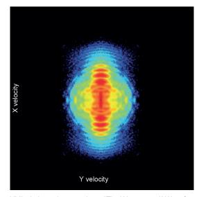
VMI of photoelectrons from ATI of Xe at 1x10<sup>14</sup> Wcm<sup>-2</sup>. With permission from MBI, Berlin.
