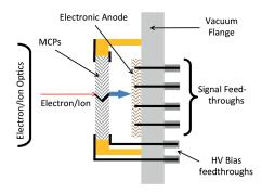
**Imaging Electron Anode Configuration**
