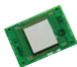
Pyrocam IIIHR 12.8X12.8mm array
