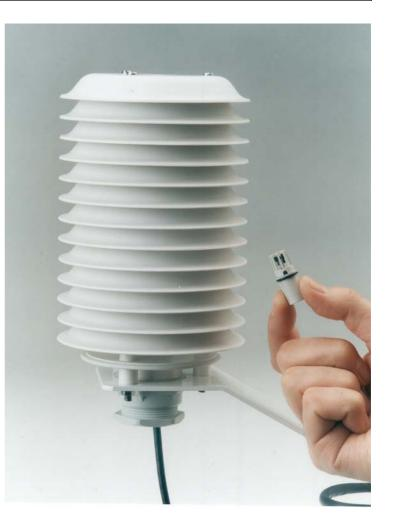
The RH and air temperature sensing elements are contained in a plug-in module. The module is interchangeable and can be replaced at routine maintenance intervals.
