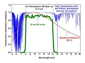
Spectral response of SI series infrared radiometers. Spectral response (green line) is determined by the germanium filter and corresponds closely to the atmospheric window of 8-14  $\mu m$ , minimizing interference from atmospheric absorption/emission bands (blue line) below 8  $\mu m$  and above 14  $\mu m$ . Typical terrestrial surfaces have temperatures that yield maximum radiation emission within the atmospheric window, as shown by the blackbody curve for a radiator at 28 C (red line).
