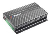
This datasheet covers four (4) product series (i.e. FA, FV, XA and XV series) of High-Precision Universal 2- and 4-Channel LED Controllers with External Triggers and 0.1mA Current Resolution, which currently include 8 models in total. All FA/FV/XA/XV LED controllers have 0.1mA current resolution, and a maximum current of 100mA in DC mode and 350mA in pulse mode.
