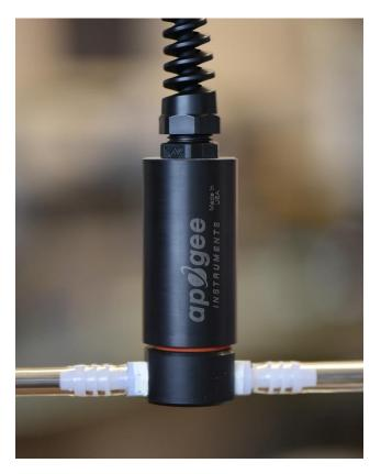
Note: To facilitate the most stable readings, sensors should be mounted vertically, with the opening pointed down and the cable pointed up. This orientation allows better contact between the electrolyte and signal processing circuitry.
