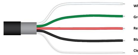
White: Positive Heater Power Green: Negative Heater Power Red: Power In (4.5 to 24 V DC) Black: SDI-12 Data Line Clear: Ground (shield wire)
