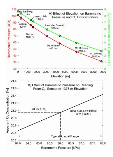
A) Barometric pressure and absolute oxygen concentration at 20 C as a function of elevation. Equation (6) was used to calculate barometric pressure.
