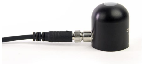
Cable connectors are attached directly to the head.
