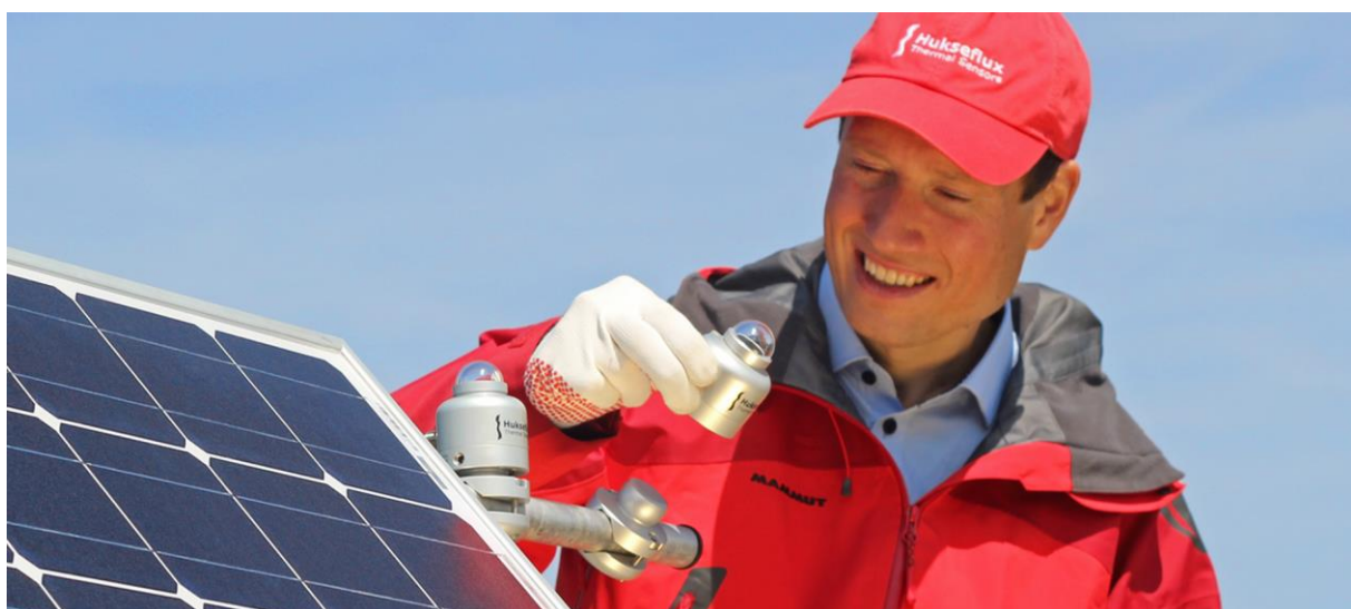
Figure 0.2 Two SR05-D1A3-PV digital second class pyranometers, of which one measuring in Plane of Array, replacing PV reference cells
