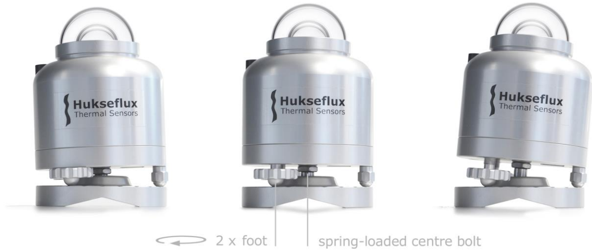
Figure 5.3.1.5 SR15 locked on its optional levelling mount: by fastening (on the left) or loosening (on the right) SR15's two adjustable feet, SR15 can be levelled, judging by the bubble level. SR15's static foot remains fixed. In all cases, ensure the legs of SR15 fit into one of the small ledges of the levelling mount. Locking is in place, when the nut is turned all the way against the bottom plate of SR15.
