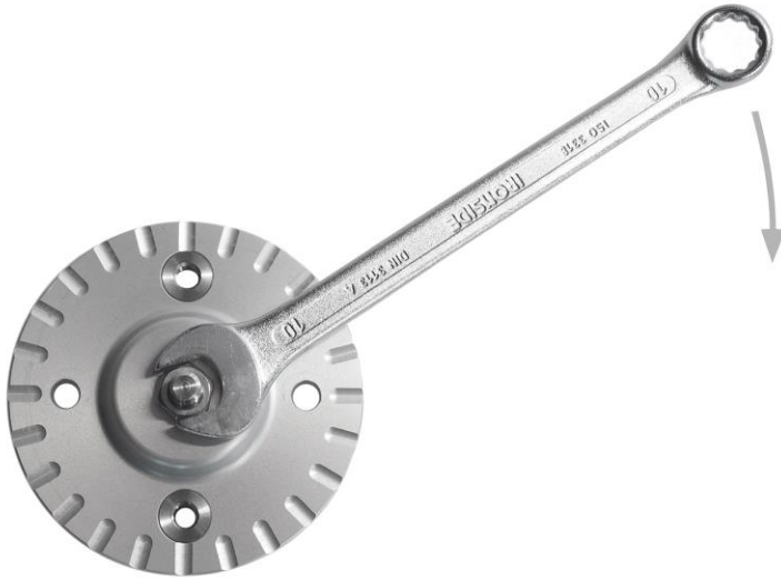
Figure 5.3.1.3 SR15 levelling mount seen from above: (un)locking with a 10 mm spanner
