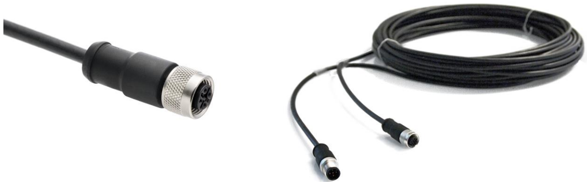
Figure 0.6 On the left the SR15 cable with M12-A female connector on sensor end, stripped over 0.15 m and conductors with ferrules. Its length is 5 metres standard and available in 10 and 20 metres too. On the right the optional Hukseflux extension cable with connector pairs, with male and female M12-A connectors, available in 20 metres
