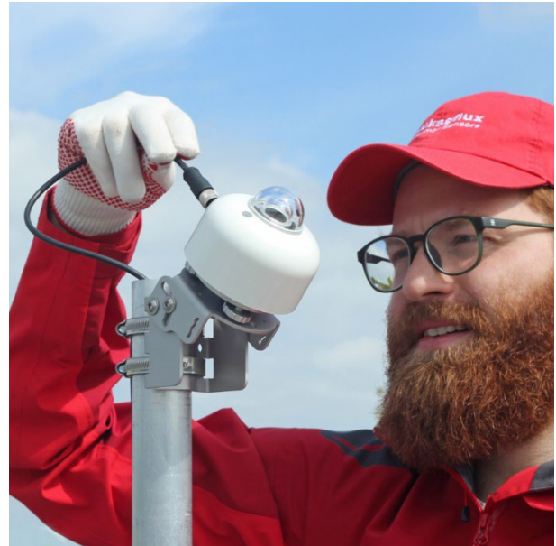
Figure 9 PMF01 pyranometer mounting fixture can be used for easy installation of a pyranometer in Plane of Array for PV system performance monitoring.
