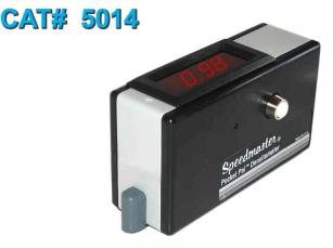
The S **\*** SM-14 is accurate to+/- .02 from 0.00 to 4.00 Optical Density. The push button switch "wakes up" the Pocket Pal to give a stable reading in just 1 second. Simply place film on your viewer, put the SM-14's "EASY READ" probe on the area to be read then push the read button.
