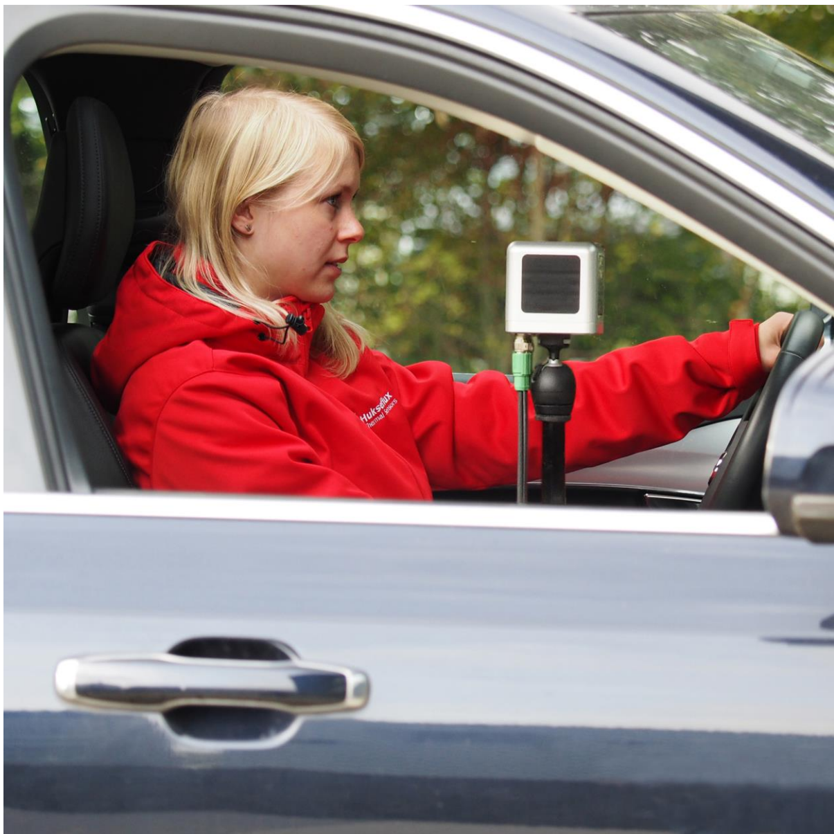
Figure 0.4 TCOM01 applied in car passenger comfort testing
