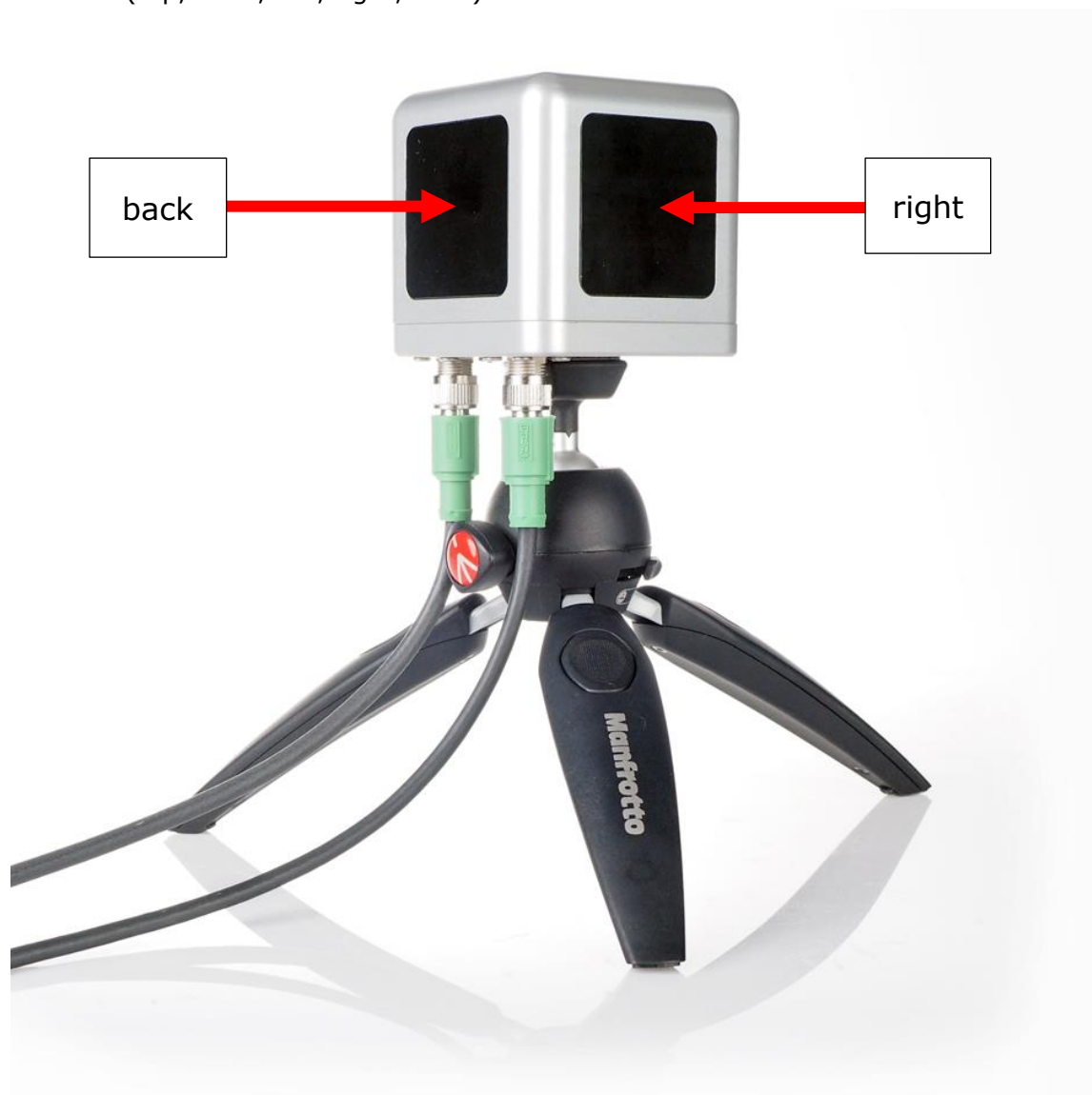
Figure 2.2.1 TCOM01 consists of an aluminium body (1) that is stabilised at a user adjustable 33 °C using an internal heater. It is equipped with five FHF01 heat flux sensors (2) with a black absorptive coating and an internal sensor body temperature measurement
