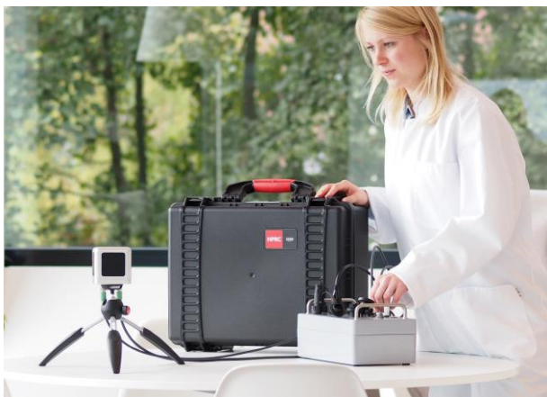
Figure 2 a complete system for measuring thermal comfort
