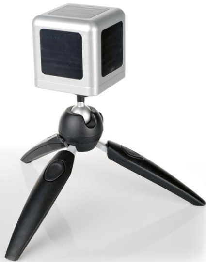
Figure 1 the TCOM01 sensor body on a tripod. The TCOM01 is meant for surveys of thermal comfort as experienced by the human body. It is equipped with 5 x heat flux sensor (black surfaces) and a sensor body temperature sensor. Heater power, ambient temperature and relative humidity are measured in the accompanying MCU (Measurement and Control Unit)
