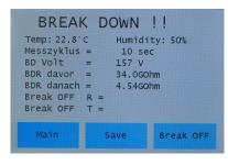
The "BREAK DOWN!!" menu opens automatically after a break-down occurs.
