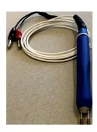
For surface resistance measurements on small packages (e.g. SMD blister tapes, conveyor belts, thermoforming trays, etc..)
