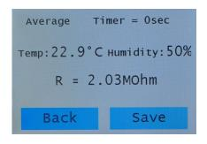
In the first row you see the Measure mode and timer counts down to zero when the measured value is stabile. In the 2<sup>nd</sup> row temperature and humidity In the 3<sup>rd</sup> row the measure value
