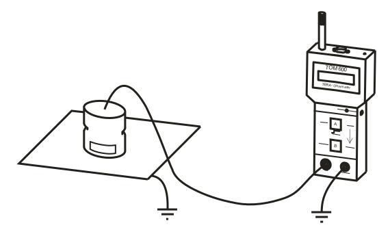
A ring measurement electrode for measurements according to DIN EN 61340-2-3 is also available as accessory.
