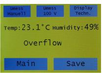
If the battery voltage drops below 4. 4 V, the current values are highlighted. (yellow)
