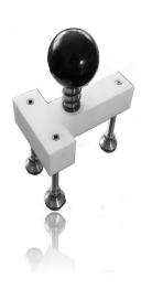
Measuring electrode - Tripod with conductive rubber pads and contact pressure 50 Newton
