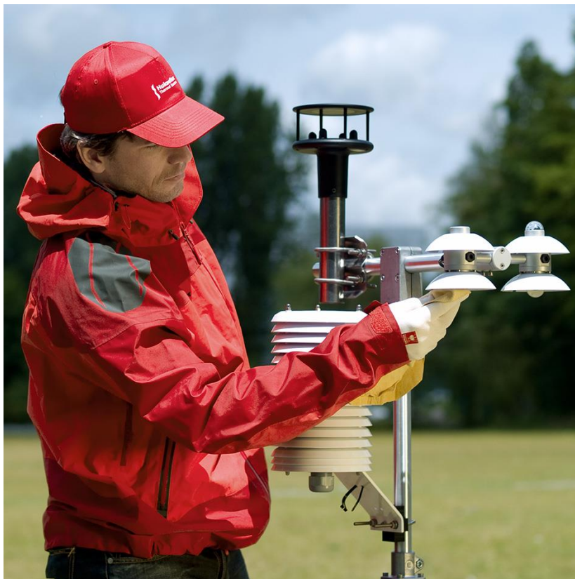
Figure 4.1 Typical meteorological surface energy balance measurement system with TP01 installed under the soil.
