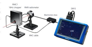
The RMC1 chopper should be mounted with the side marked "THIS SIDE TOWARD SENSOR" facing the RM9. The side of the chopper blade facing this direction has a low emissivity surface to minimize measurement artifacts that could be caused by thermal signal from the chopper blade. The other side of the blade faces the light source and has an absorptive black coating to minimize stray reflections.
