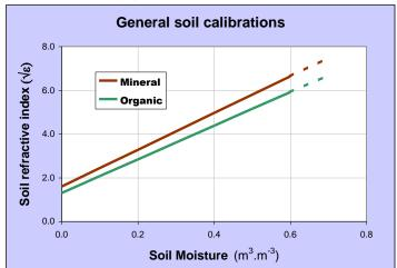
In DeltaLINK, the soil type for a WET150 logging program can be selected from a drop-down in the properties panel on the right of the program editor window, under the calculation section. This auto-populates the  $\boldsymbol{a_0}$  and  $\boldsymbol{a_1}$  values for the water content (theta) calculation.
