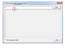
Once the SDI-12 Transparent Mode Terminal is open, the GP2 behaves like a transparent serial link between SDI-12 sensors and the PC.
