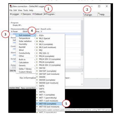
Illustration: showing steps in the creation of a WET150 soil moisture sensor measurement type in a GP2 program.
