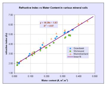
You can see from this graph that the accuracy of the water content measurements would be improved by using a different calibration for each soil. However, the improvement would be small (typically 2 or 3%), so a generalised "mineral" calibration is appropriate for a good range of agricultural soils.
