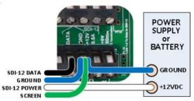
Ensure there is a fuse or other protection in-line with this external power source in case short-circuit faults develop on the SDI-12 network.
