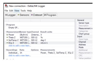
Illustration: DeltaLINK, GP2 Program tab with a default Recording interval set to 1 hour for each of the defined Measurements.
