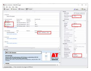
Showing the addition of address Z to the WET150 Measurement names
