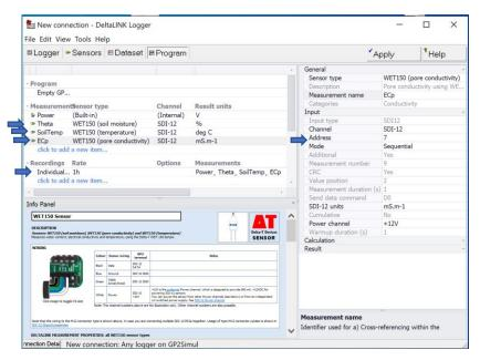
Illustration showing three sensor measurement types added to take readings from a single WET150, for soil moisture, pore water conductivity and temperature. These all have the same SDI-12 address, which in this example has been changed to 7 from the default 0 address. The default measurement period of 1 hour for all readings can be also seen.
