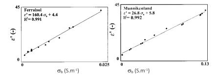
Figure 1 - Examples of the relationship between  $\varepsilon'_b$  and  $\sigma_b$ , showing the offset  $\varepsilon'_{\sigma_b=0}$  for two different soils.
