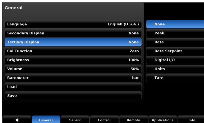
Figure 7.1.2 - Secondary and Tertiary display
