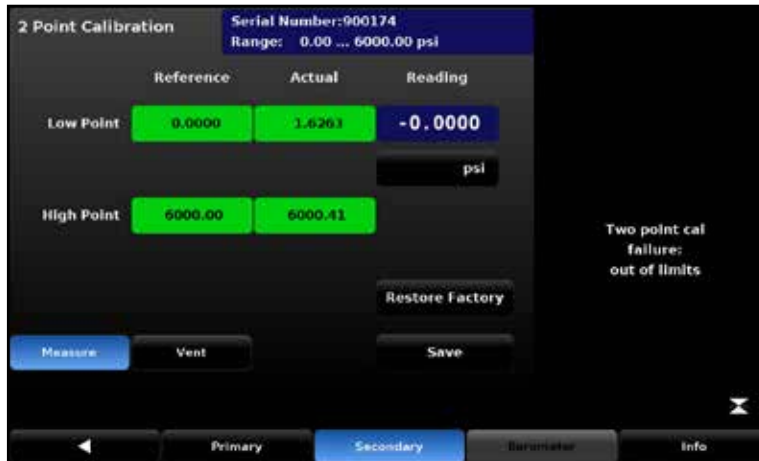
Figure 6.4.2.5.2-9 – ‘2 Point Calibration Failure’]
