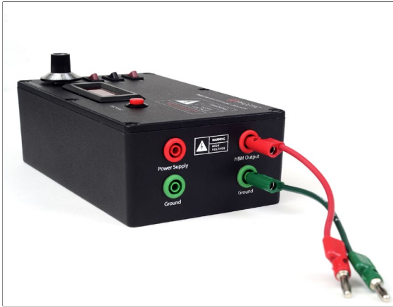
Figure 1. Connect the 510-054 red lead to the HBM Output connector on the PDS-510
